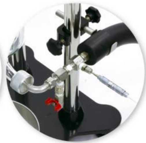
In-line Pt100 Sensor connected to inlet of the thermal jacket
